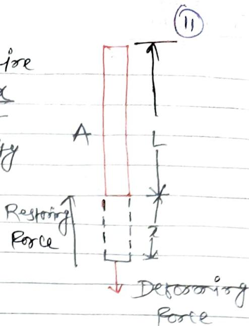
$\therefore$  This force is a variable force. So, work done by variable force to elongate the wire by amount  $x$ ,
