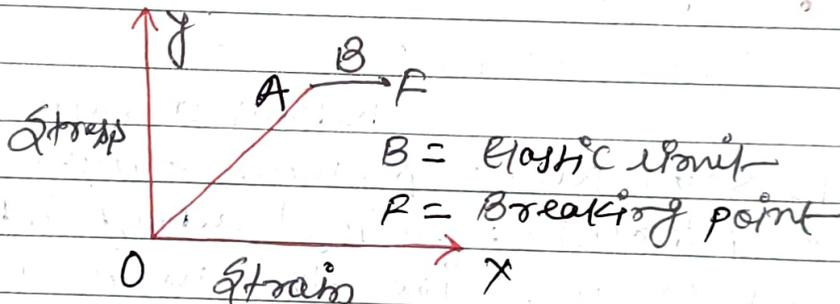
③ Elastomers :-> These are those materials for which stress and strain variation is not straight line within elastic limit. The elastic region is very large. These materials do not obey Hooke's law and such materials have no plastic range. e.g -> Rubber, The elastic tissue of organs etc.
