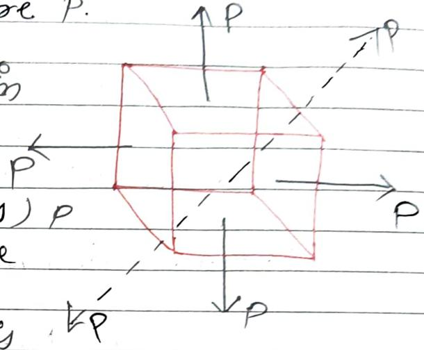
The pressure (stress)  $P$  which is along the  $x$ -direction will elongate the  $x$ -axis and compress  $y$  and  $z$ -axes.
