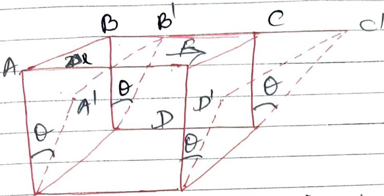
It is the ratio of tangential stresses to shear strain
